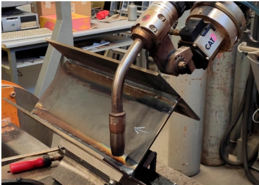
Figure 2. Metal-Core Arc Welding Experimental Setup, (Perić M., and et al. 2023).
