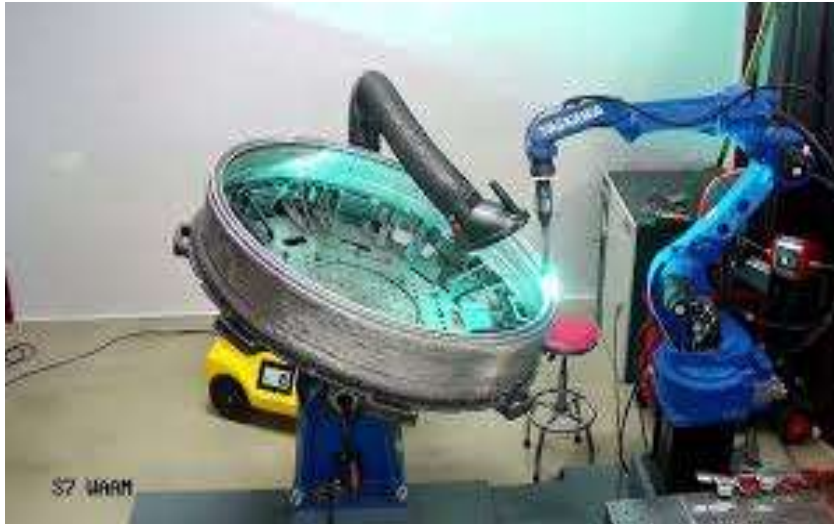
Figure 4. Robotic Arm with Wire Arc Additive Manufacturing (WAAM) (yaskawa.com.tr, 2025).
