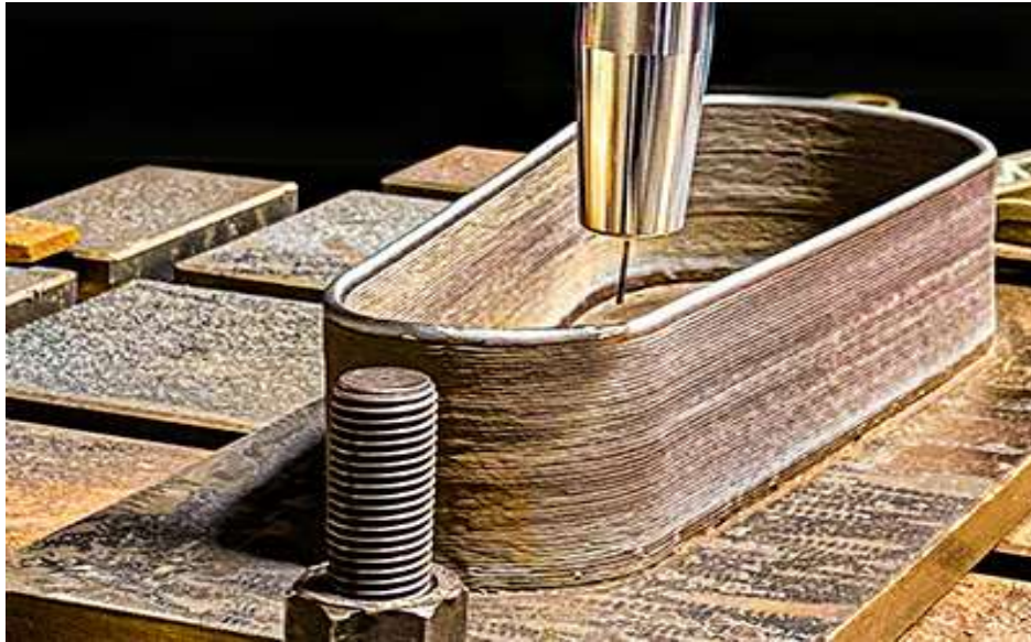
Figure 3. Wire Arc Additive Manufacturing (WAAM) and industrial applications (gedik.com.tr, 2025).
