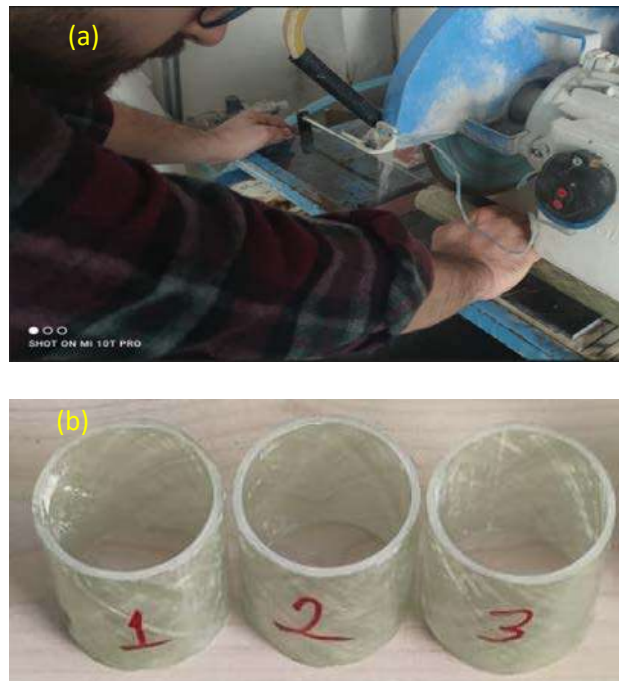
Figure 1. (a) Sample ceramic cutting machine (b) Sample specimens prepared for burning test
