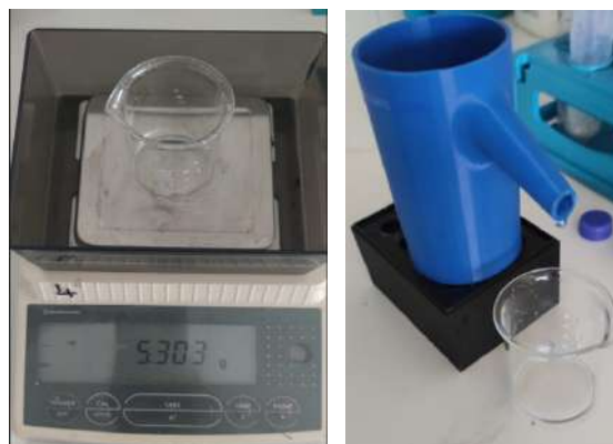
Figure 2. (a) Shimadzu precision balance (b) Archimedes cup for measuring sample volume
