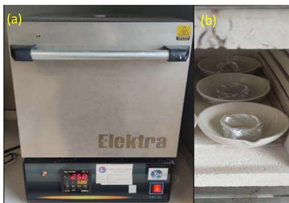
Figure 3. (a) Elektra brand muffle furnace (b) Sample images after incineration test
