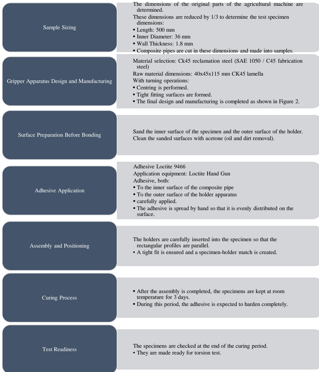
Figure 5. Test Specimen Preparation Algorithm for Torsion
